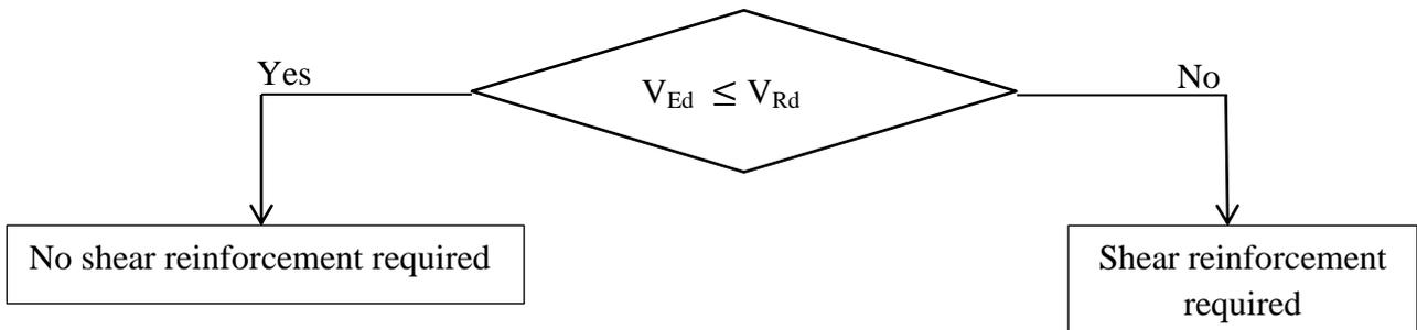
**Fig.3 Flow-chart for shear reinforcement**
