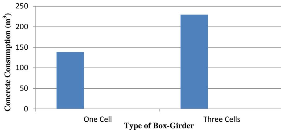
Fig.10 Graph Showing Comparison between Concrete Consumption and Types of Box-Girder
