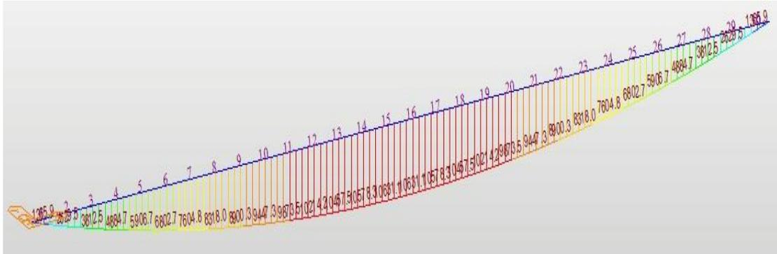
**Fig.8 Beam Diagram Single cells Concrete Box Girder**
