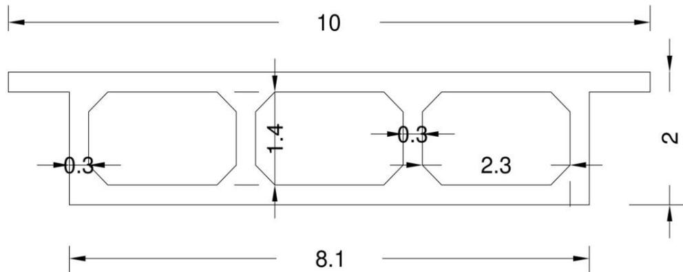
**Fig.1 Cross-sectional details of 3 cells Concrete Box Girder (all dimension are in meter)**
