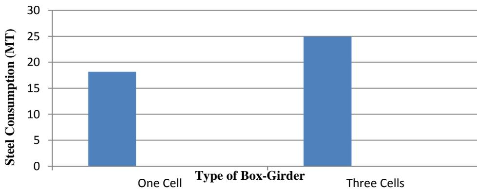
Fig.11 Graph Showing Comparison between Steel Consumption and Types of Box-Girder
