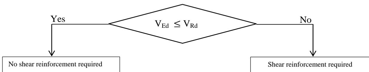
Fig.7 Flow-chart for shear reinforcement
