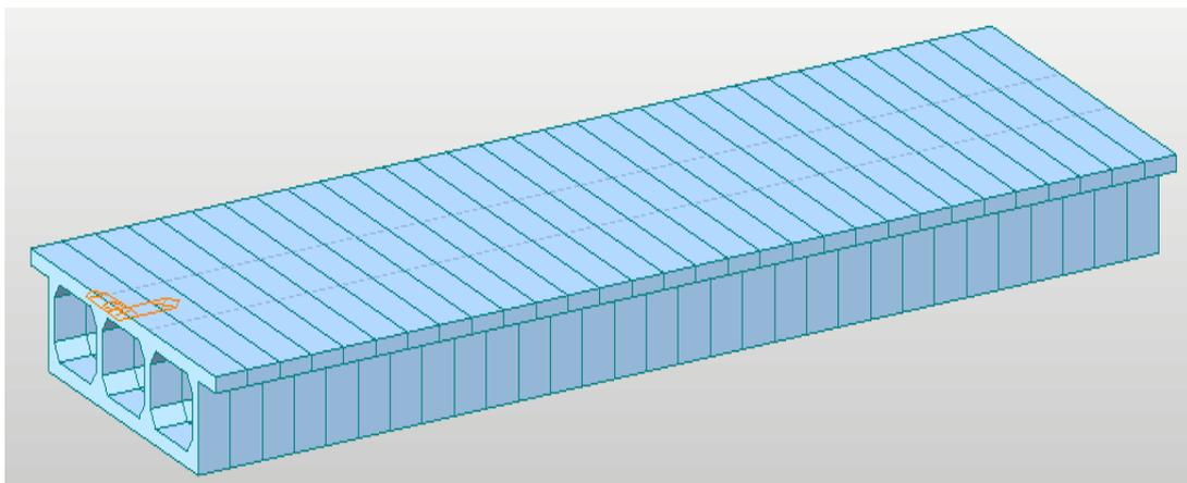
**Fig.2 Perspective view of 3 cells Concrete Box Girder**
