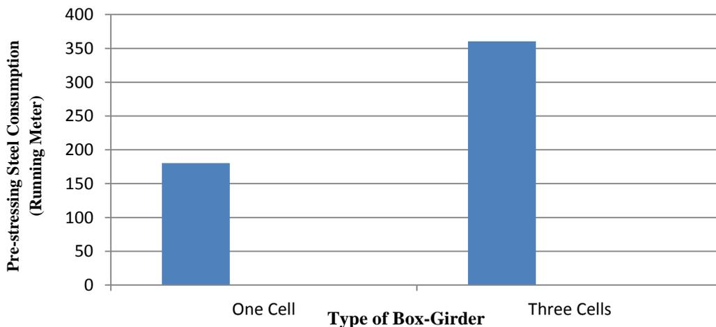
Fig.12 Graph Showing Comparison between Pre-stressing Steel Consumption and Types of Box-Girder
