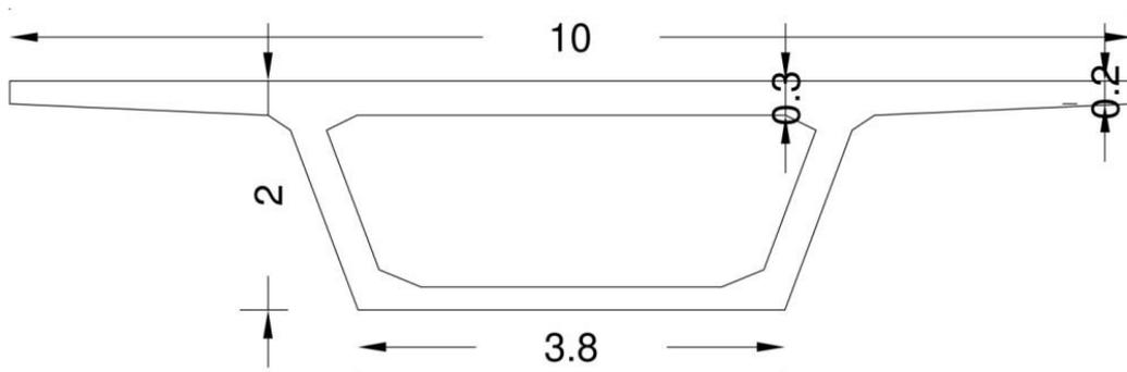
Fig.5 Cross-sectional details of Single cells Concrete Box Girder (all dimensions are in meter)
