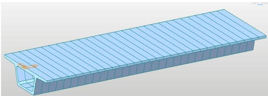
Fig.6 Perspective view of Single cells Concrete Box Girder
